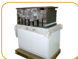
Actual photo during Cabinet Load Testing
