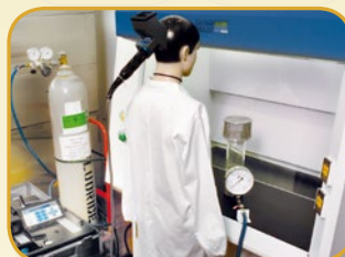
Tracer Gas (SF 6 ) Containment Test
